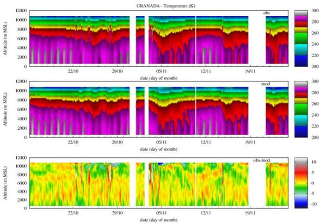
Fig. 2. Example of collocated temperature profile observations from MWR (top) and background simulations from Arome-WMed (middle). Observation-background (O-B) differences are shown in the bottom panel (Granada, Spain).
