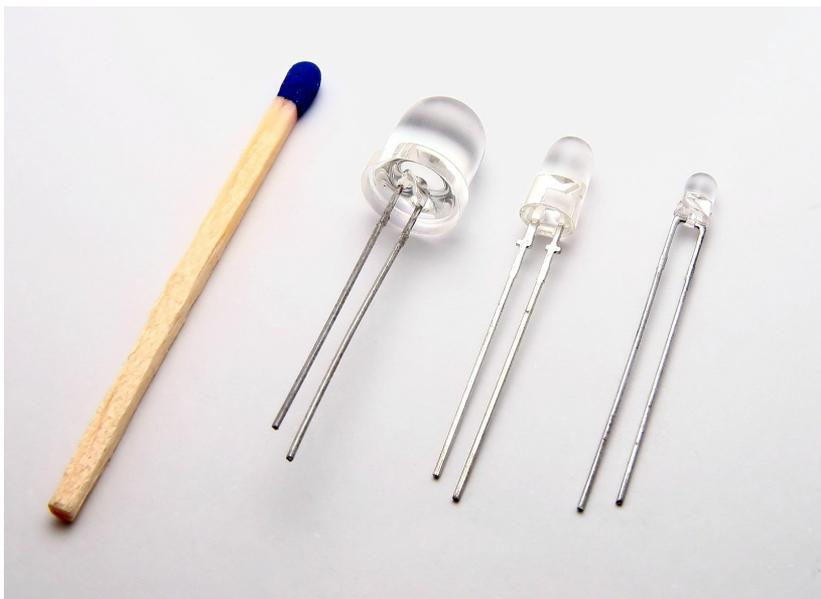
**Figure 3-1.** LEDs in 8 mm, 5 mm, and 3 mm sizes.
